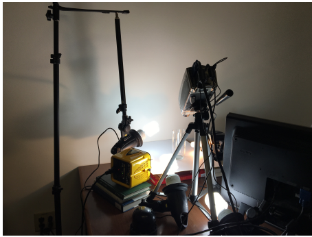
Lighting placement for filming, with Olympus I-Speed from initial attempts, and approximate locations of lights shown
